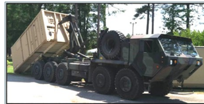
MWMSS System container unloading after transport.
